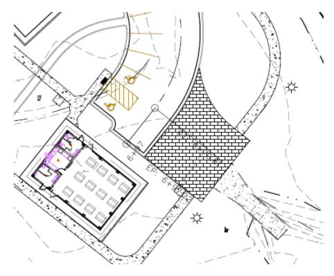
2. The plans have been amended to include the placement of approximately 150 feet of 4" PVC conduit under the sidewalk at locations established by the engineer. Most crossings will be placed in 10 to 20 feet long lengths. The Schedule of Items has been adjusted to include this item of work.
